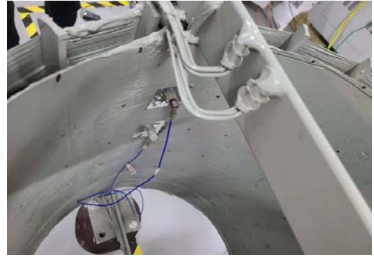
图 9 电抗器内层包封的振动测量 Fig. 9 Vibration measurement of the inner layer of the air-core reactor
