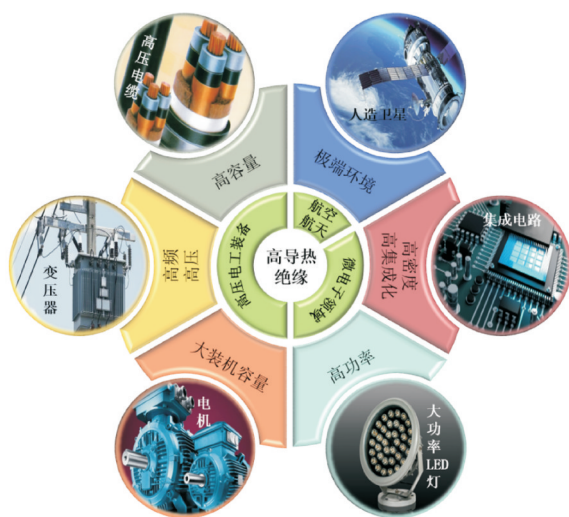
图1 高导热复合绝缘材料应用领域 Fig. 1 Applications of high thermally conductive composite
